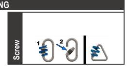
WARNING! If the lanyard is equipped with SCREW locking carabiners, please make sure that the gate is fully closed and tightened correctly, before using it! Note: SCREW locking carabiners shall NOT be used at workplaces where the user must connect/disconnect frequently! If the lanyard is equipped with AUTO-LOCK, TRI-LOCK or TWIST-**LOCK** carabiners, make sure that the gate is fully closed and secured before use.
